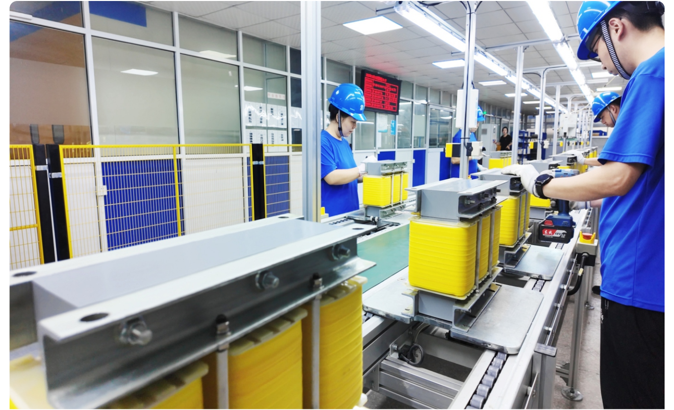
LV reactors assembling
