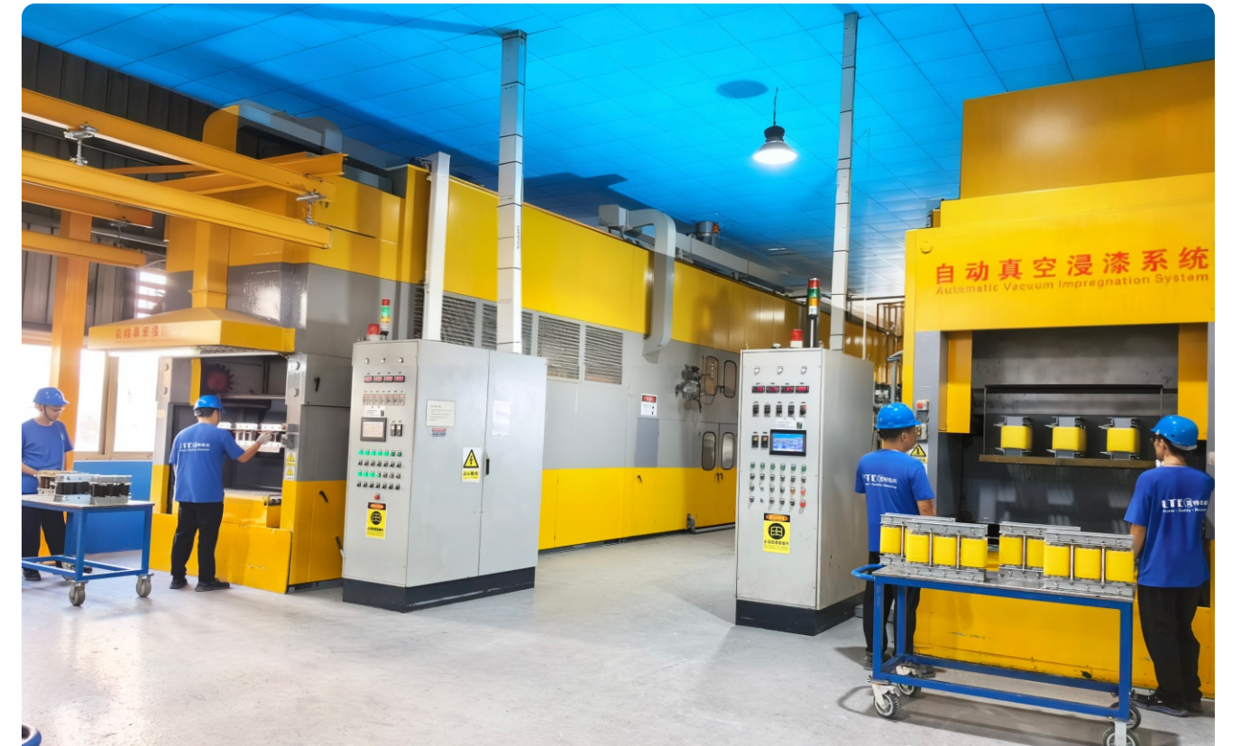
Automatic vacuum impregnation system
