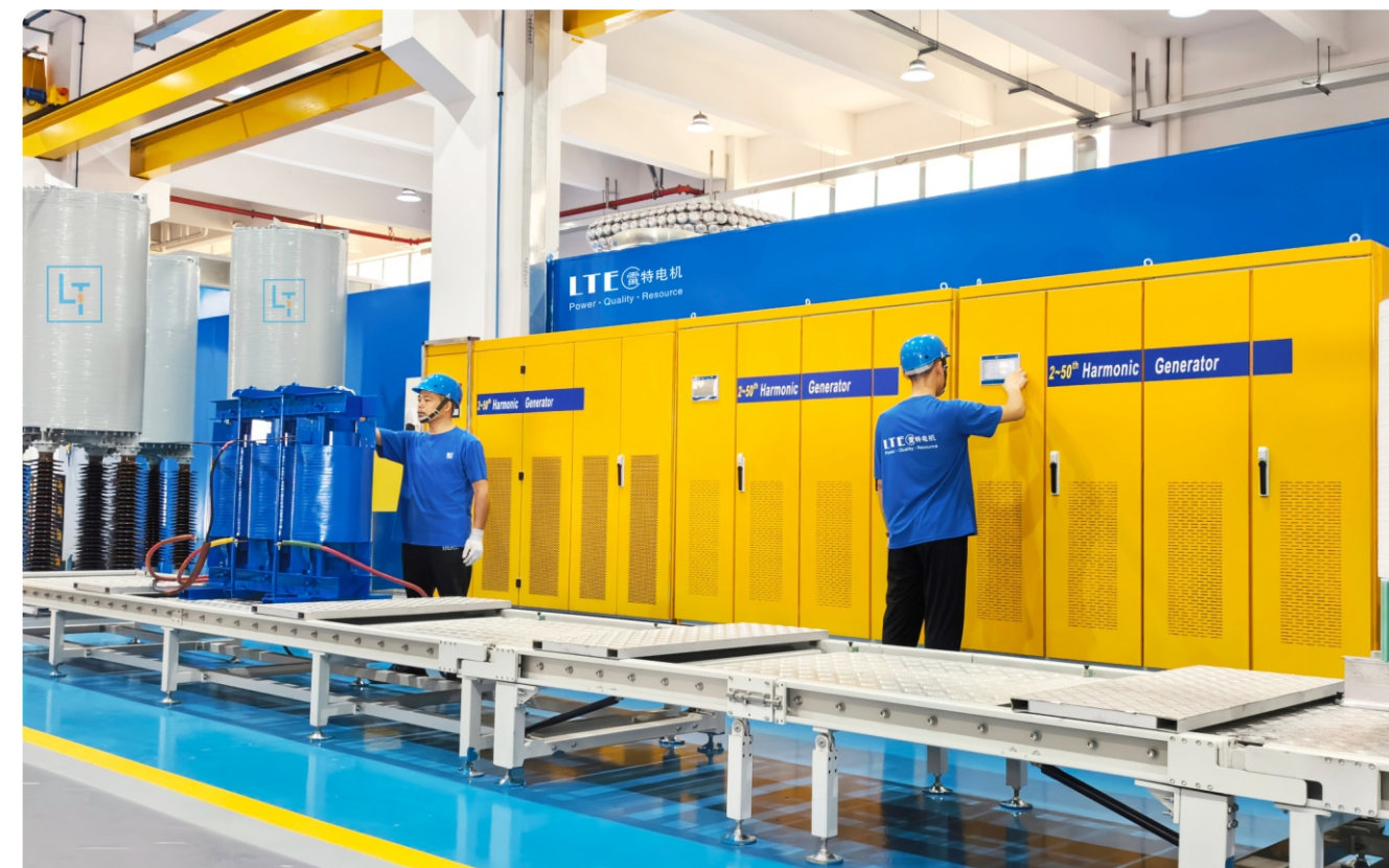
Harmonic filter reactor testing
