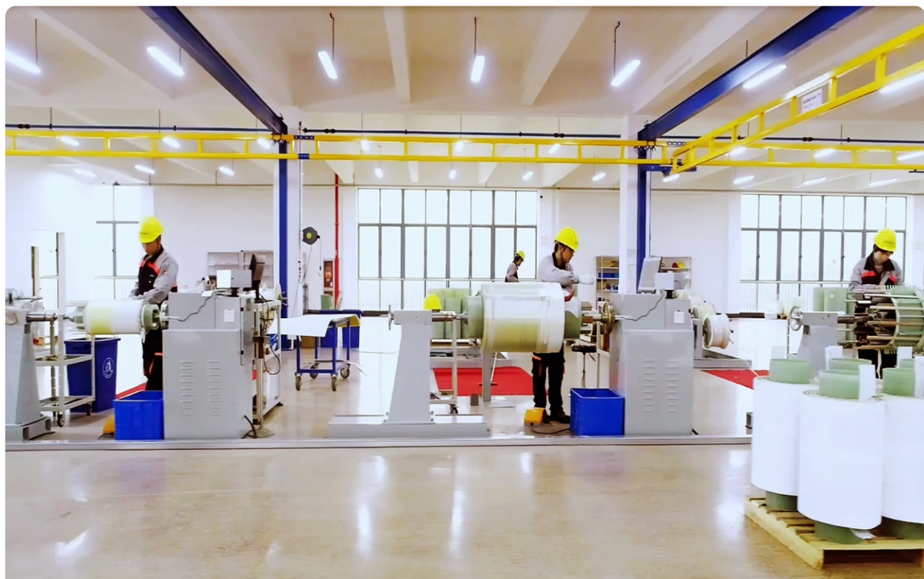
Medium voltage winding
