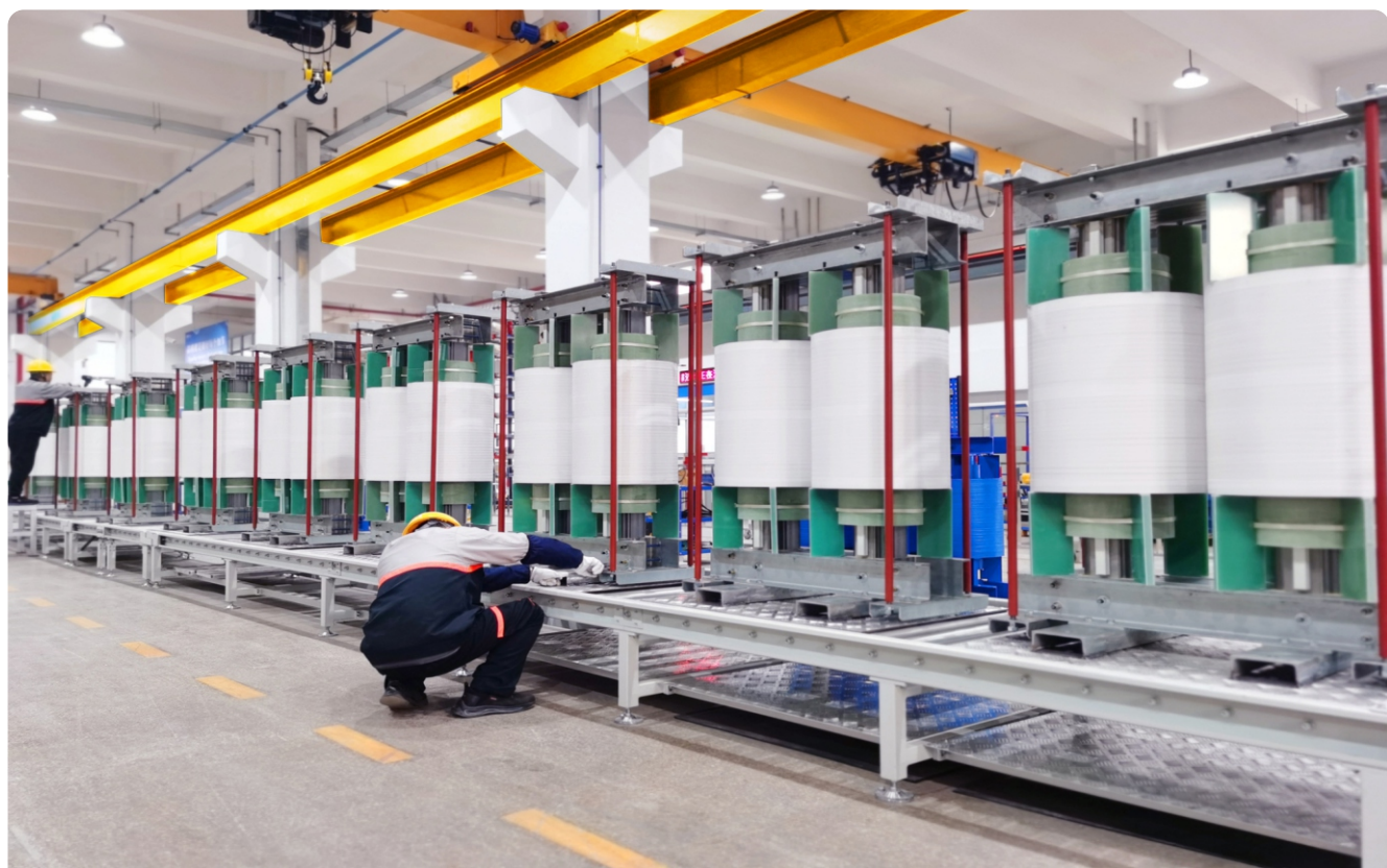
MV reactors assembling
