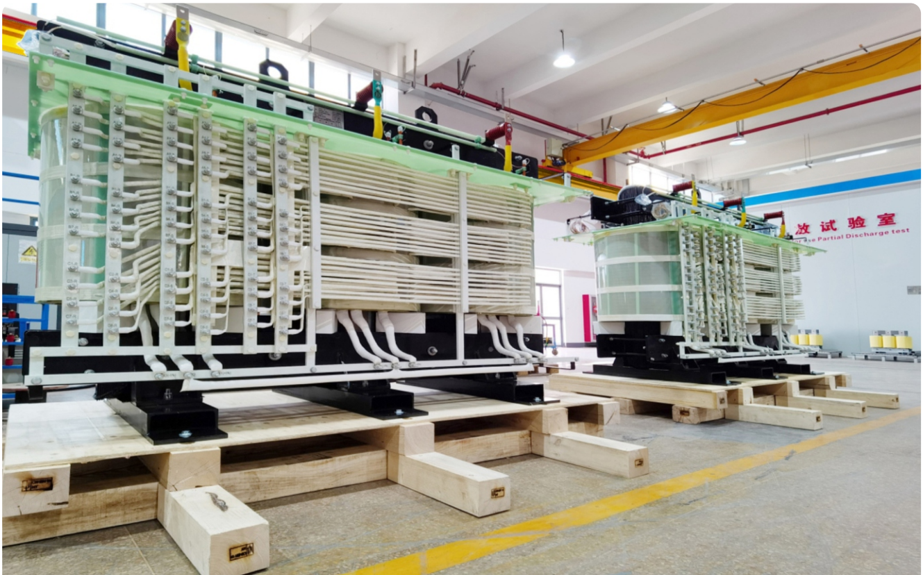
6000 kVA Phase-shifting transformers
