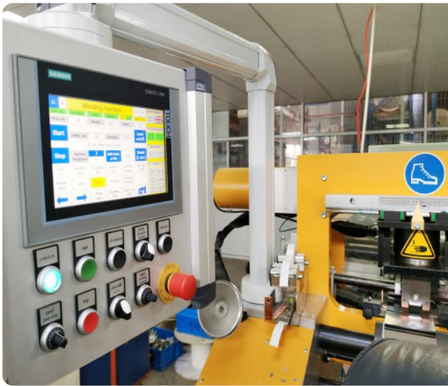
Copper & Aluminum cold pressure welding
