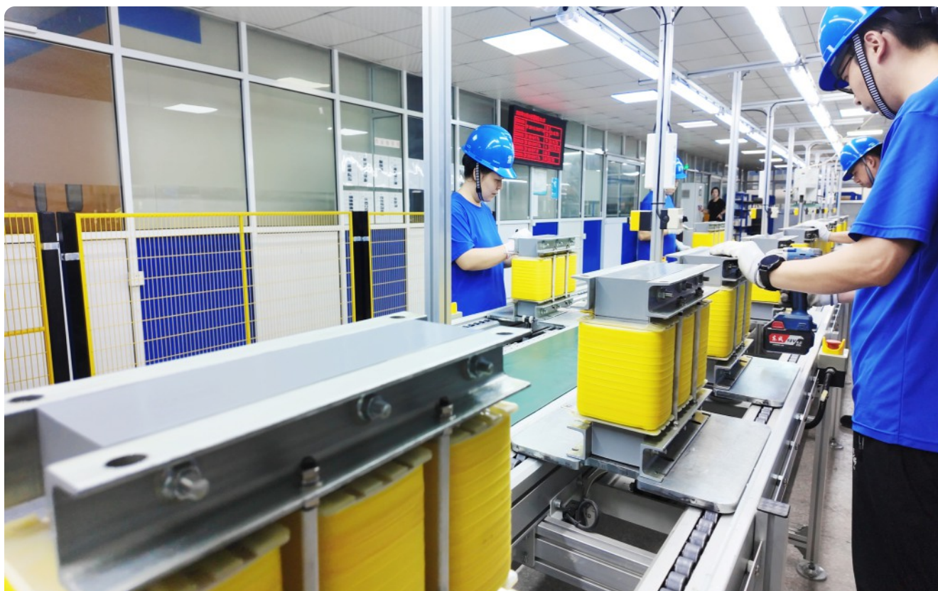
LV reactors assembling
