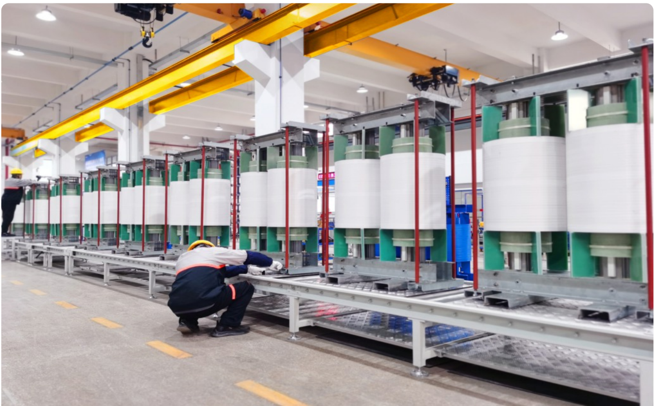
MV reactors assembling
