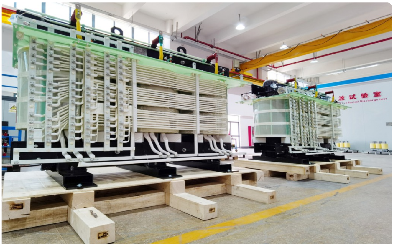
6000 kVA Phase-shifting transformers
