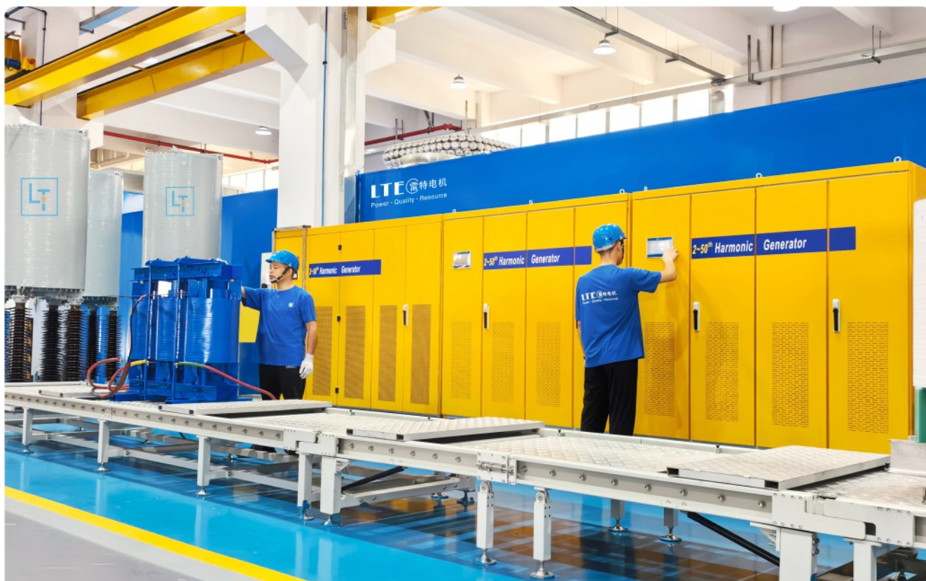
Harmonic filter reactor testing
