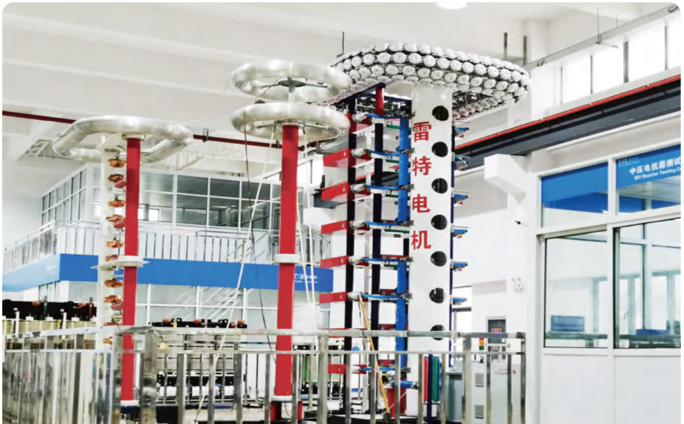
The lightning impulse equipment testing up to 1200 kV
